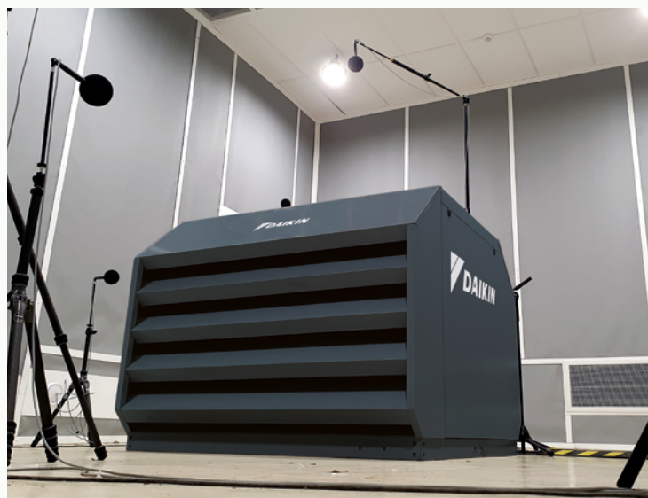
Sound power level measurement in acoustic chamber
