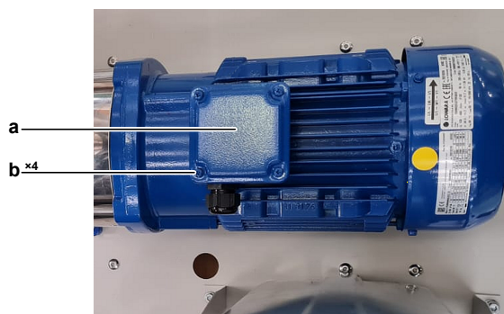
a Electrical connection box cover b Screw
