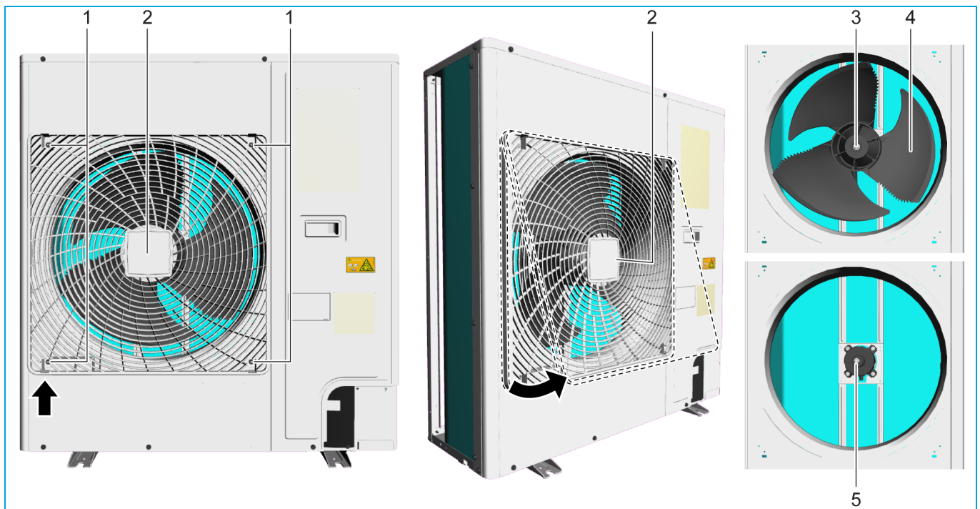
Figure 3-31: Removing the propeller fan blade assembly
